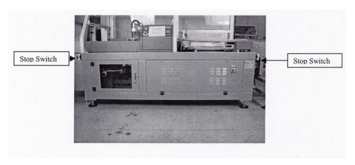
Emergency stop switch located at infeed side on PP 50 BM
