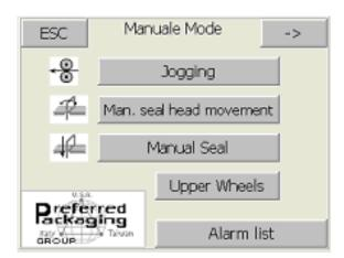
5 Press upper wheels to open side seal film drive wheels.
